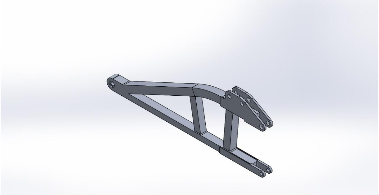
Figure 12: Trailing Arm Design in CAD
