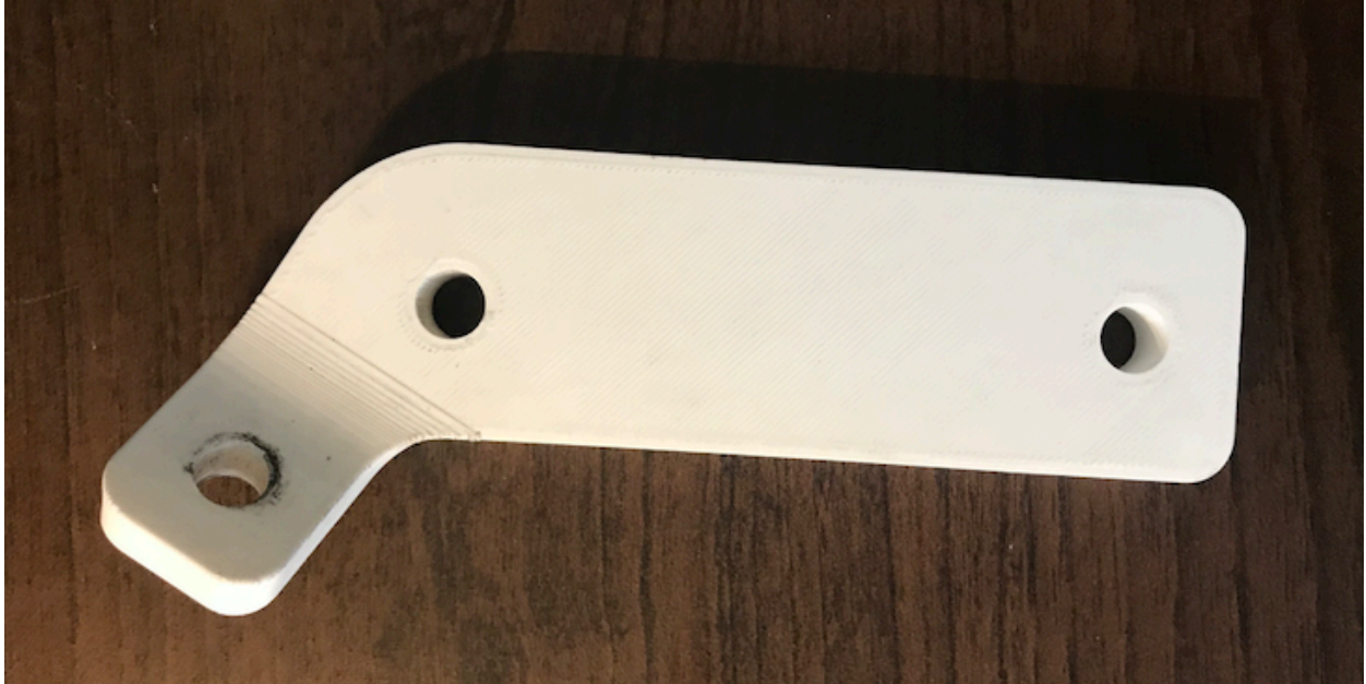
Figure 1. Top View of Steering Attachment Link
