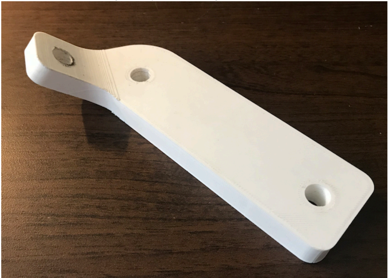
Figure 2. Isometric View of Steering Attachment Link
